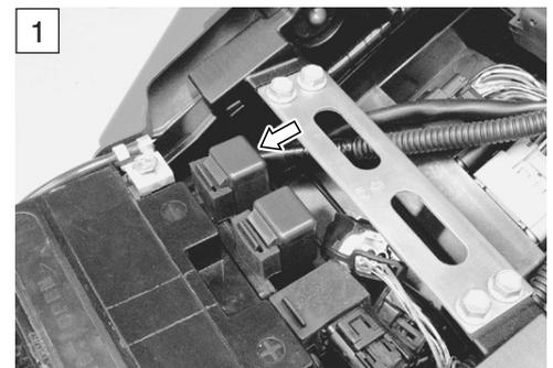
Is the cooling fan relay OK?
