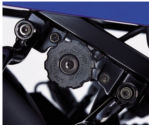
Hydraulic spring preload adjustment system
