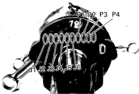
**Crankshaft main journal and crank pin bearing selection**
