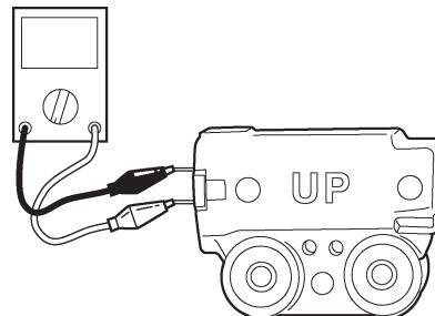
**Lean angle cut-off switch voltage**
