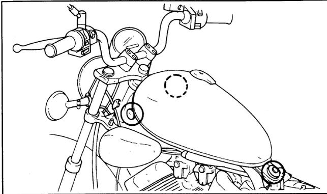
3. Lift the front of the sub fuel tank upward and position it away from the air filter. (Do not remove it.)
