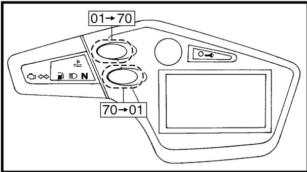
4. Press the “SELECT” button to select the CO adjustment mode “Co” or the diagnostic mode “dIAG”.
