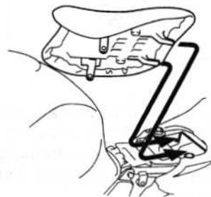
To reinstall the seat, slide the seat hook into the seat hook retainer on the frame and tighten the bolts securely.
