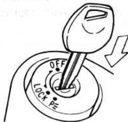
Align the lid hole position to the key hole position when inserting the key.
