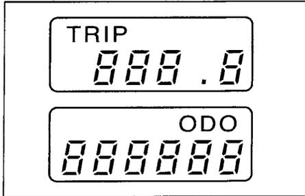
To reset the trip meter to “0”, push the “TRIP” button until it displays “TRIP”, then push it once again and hold it down for at least one second.
