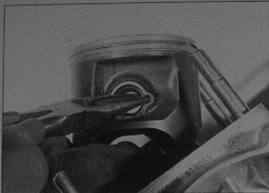
11.3 Wear eye protection and remove the circlip with a pointed tool or needle-nosed pliers
