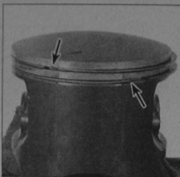
11.19b Position the ring ends on either side of the dowel pin in each ring groove (arrow)
