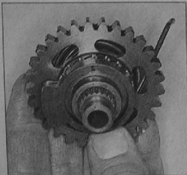
15.15 Align the ratchet punch mark with the mark on the spindle
