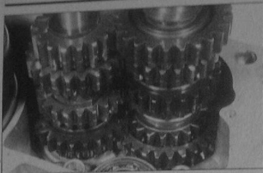
19.4 Both transmission shafts have a thrust washer on the left side
