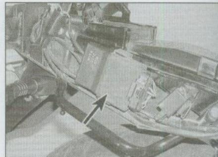
5.3 Ignition control unit (arrowed)
