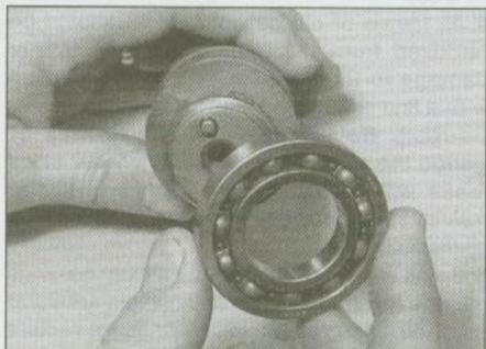
30.8 Remove the bearing if necessary
