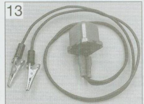
**13** A buzzer is useful for voltage checks
