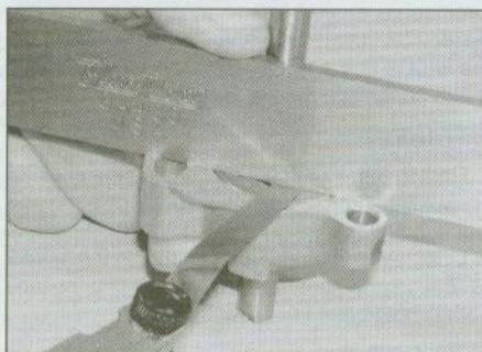
17.10 Measuring rotor end-float
