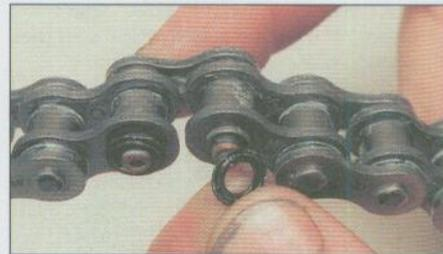
8.5 . . . install the O-rings over the pin ends . . .
