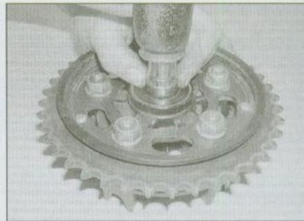
17.30 Drive out the spacer with a long socket
