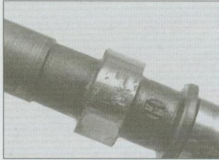
9.8a Check the lobes of the camshaft for wear – here's an example of damage requiring repair or renewal
