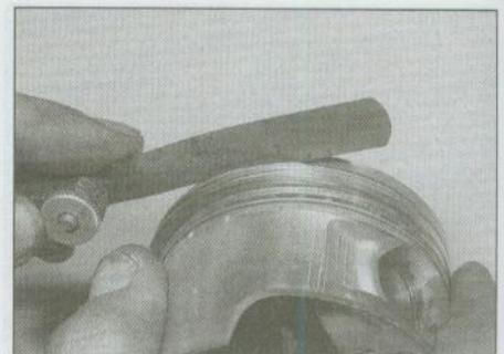
23.12 Measuring the piston ring-to-groove clearance with a feeler gauge
