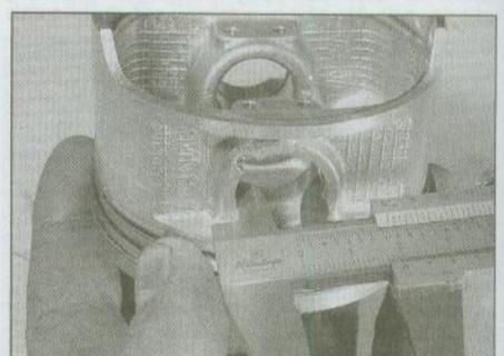
23.14b Measuring the pin bore in the piston
