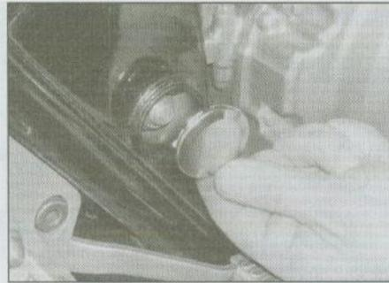
12.8a Remove caps and remove the nut from the right side . . .
