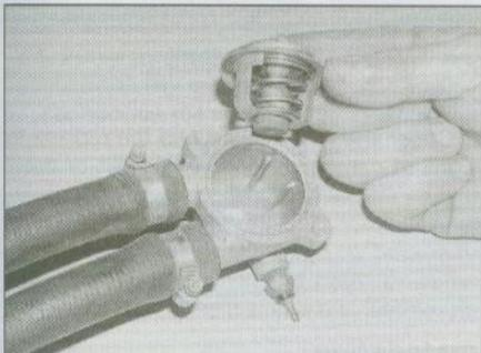
6.5c ... and withdraw the thermostat
