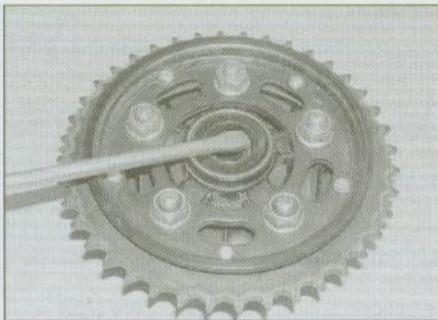
17.29 Lever out the grease seal
