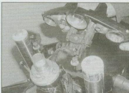
19.7 Lift the top yoke off the fork tubes
