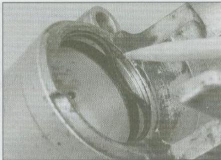
**3.10** Remove the dust seal carefully to avoid damage to the bore and seal groove
