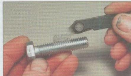
2.12 Using a thread gauge to measure pitch
