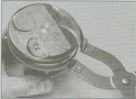
23.6a Using a ring removal and installation tool
