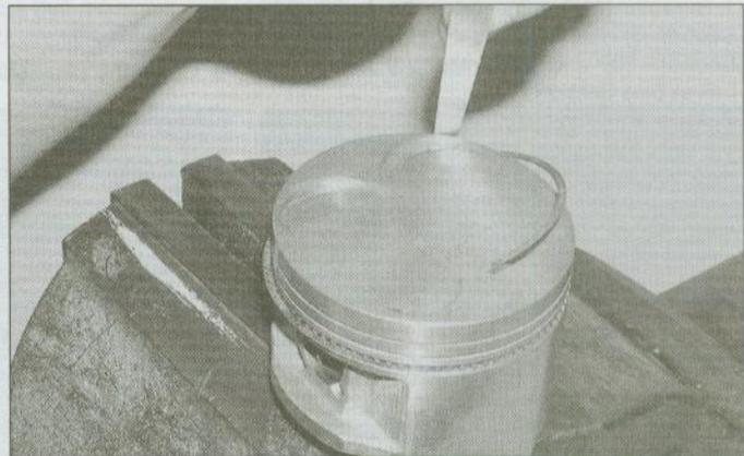
24.9b . . . then the lower and upper rails with the aid of a thin blade
