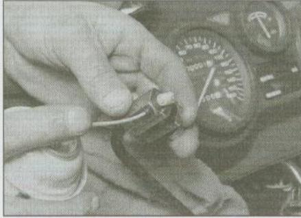
6.3a Lubricating a cable with a cable oiler clamp. Ensure the tool seals around the inner cable
