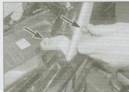
4.3 Grab rail is retained by two bolts (arrowed) on each side
