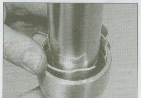
7.23 Install the oil seal retaining clip . . .
