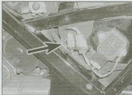
21.3 Sidestand switch wiring connector (arrowed)
