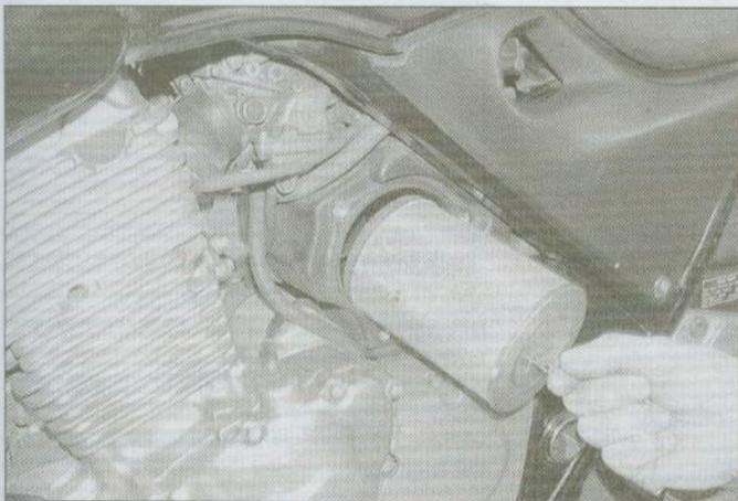
25.2 Pull the filter element out of the housing
