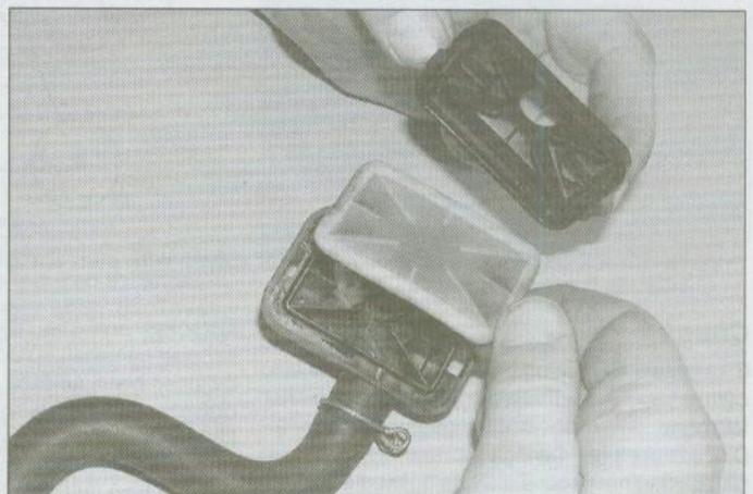
25.5 Check the condition of the sub-air cleaner element
