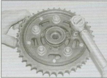
15.11b ... then unscrew the sprocket nuts
