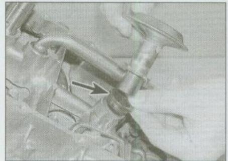
18.3 Remove the oil strainer and packing collar (arrowed)
