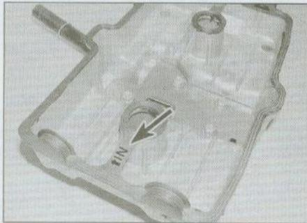
7.8c Install the cover gasket with the IN mark (arrowed) pointing to the rear
