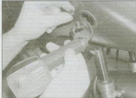
7.1b ... and withdraw the turn signal through the fairing
