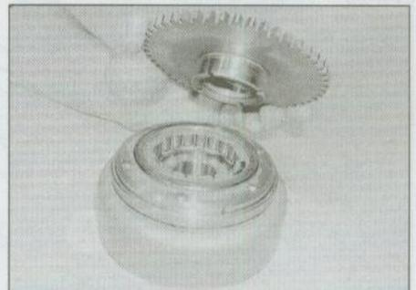
13.8 Withdraw the gear and inspect for wear or damage
