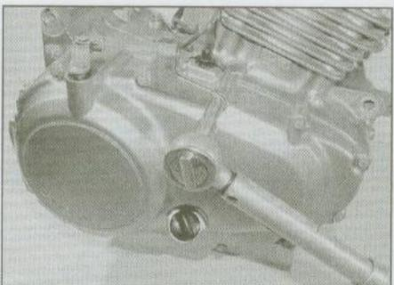
15.38b . . . then install the cover and clutch cable bracket
