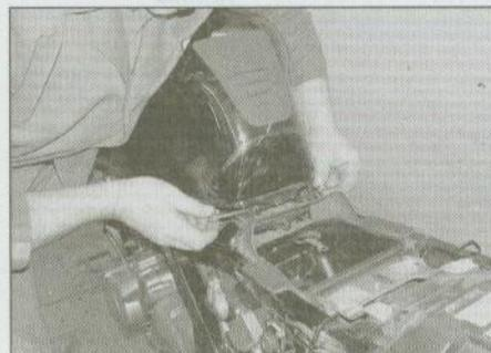
**2.4a** Unscrew the bolt at the back of the tank . . .
