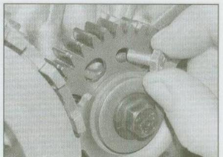
15.35 Remove the bolt locking the primary drive gear halves together
