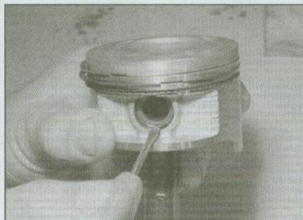
23.4a Prise out the circlip . . .
