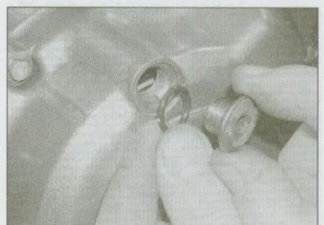
26.19 Fit new O-rings onto the plugs
