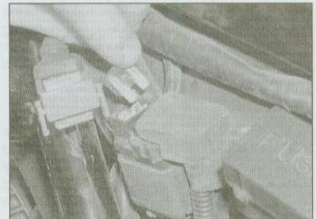
5.2b Unclip relay wiring connector to access main fuse
