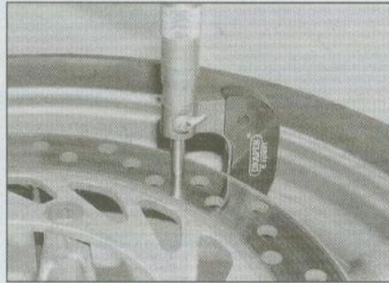
4.3b Measuring the disc thickness
