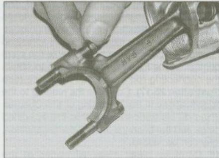
22.6b . . . before pressing the bolt into place
