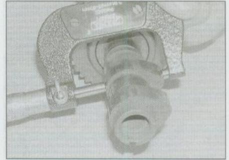
9.8b Measure the height of the camshaft lobes with a micrometer
