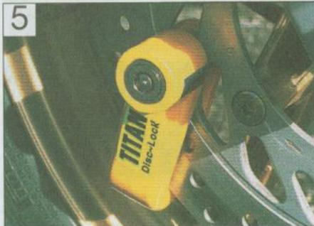
**A typical disc lock attached through one of the holes in the disc**
