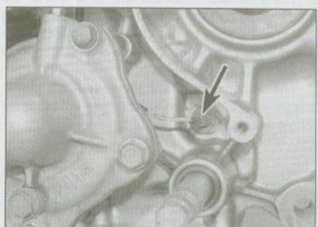
**5.17** Detach the neutral switch wiring connector (arrowed)
