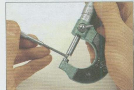
3.10 ... then measure the gauge with a micrometer
