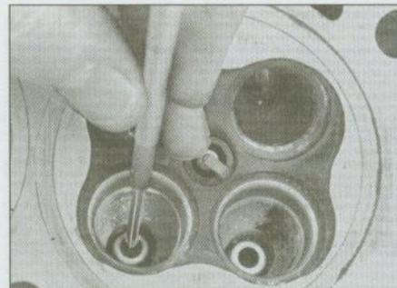
12.15b Insert a small-hole gauge into the valve guide and expand it so there's a slight drag when it's pulled out
