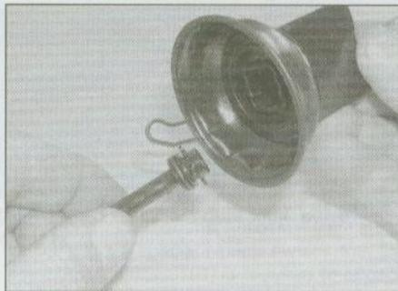
7.5b . . . and pull the holder out of the piston
