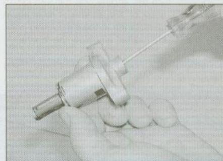
8.2b Tensioner plunger fully extended with tension released
