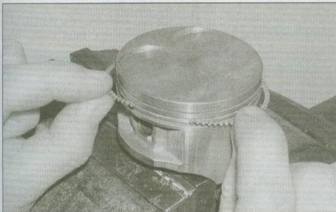
24.9a Fitting the oil control ring, first install the expander . . .
