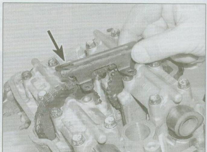
9.26b Install the camchain upper guide with reference to mark made on disassembly (arrowed)
