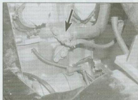
10.5 Unscrew the bolts securing the coolant pipe union (arrowed)
