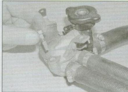
6.5a Unscrew the thermostat housing cover bolts ...
