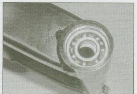
13.10 Grease both bearings before reassembly
