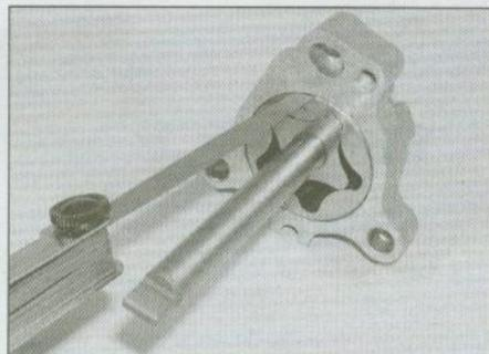
17.9 Measuring outer rotor-to-body clearance
