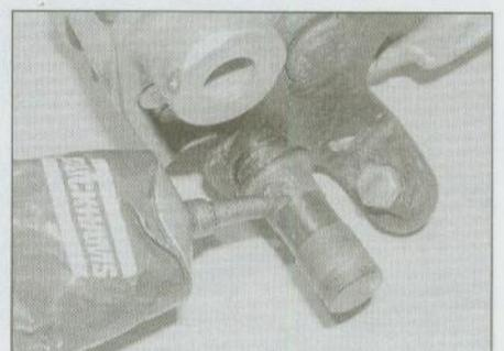
3.14 Lubricate pedal pivot before reassembly
