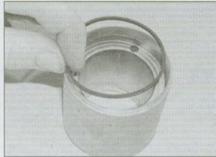
29.6 Remove the main housing and discard the O-rings
