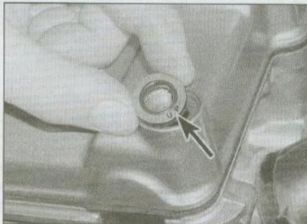
7.9a Install cover bolt sealing washers with UP showing . . .
