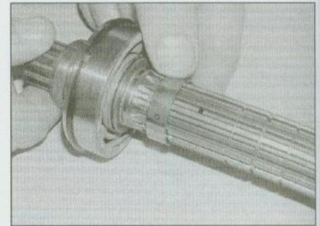
29.33a Slide on the 2nd gear pinion bush . . .
