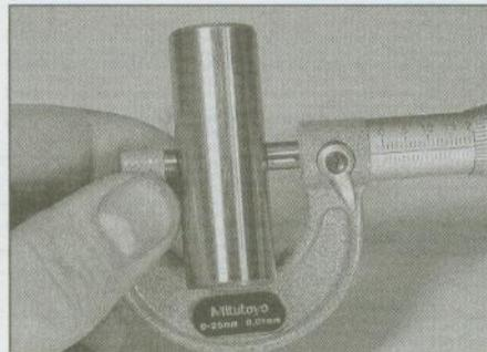
22.9b Measuring the external diameter of the pin . . .
