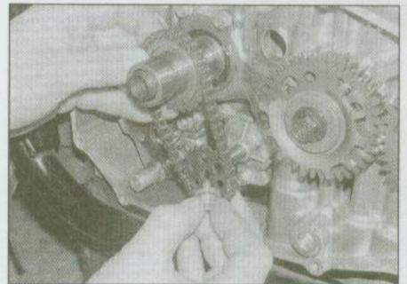
15.11b . . . and pull the sprockets and chain off as an assembly
