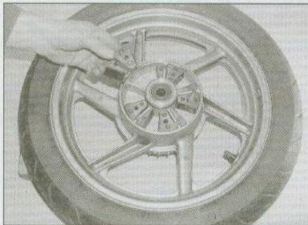
16.3 Inspect the coupling dampers for wear and deterioration
