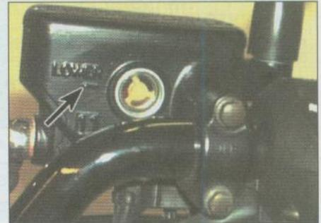
**1** The front brake fluid level is visible through the sightglass in the reservoir body – it must be above the LOWER level line (arrowed).
