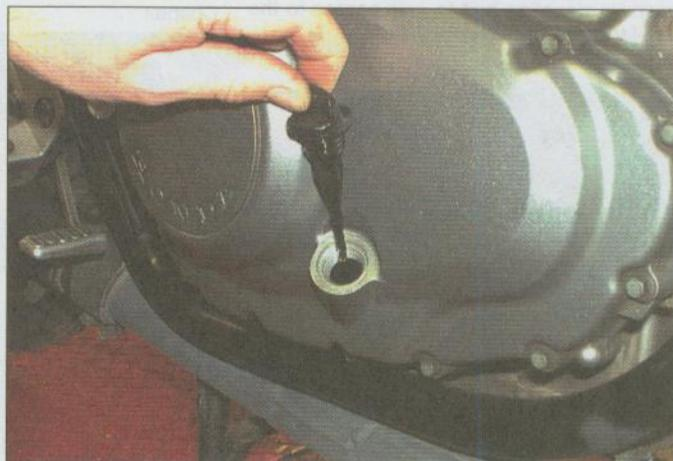
**1** Unscrew the oil filler cap (arrowed) from the right-hand crankcase cover. The dipstick is integral with the oil filler cap, and is used to check the engine oil level.
