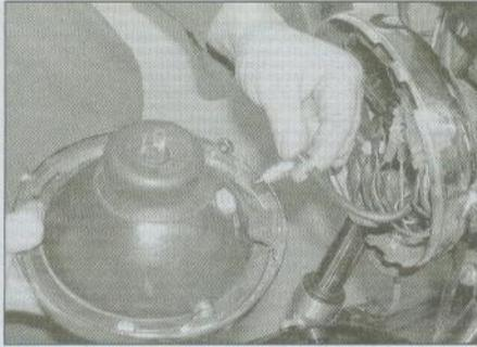
7.1c ... and pull the sidelight bulb out of its socket
