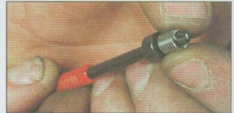
**2.28** . . . fit insert on the installing tool . . .
