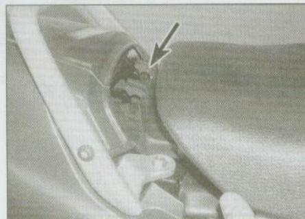
3.2 Seat hooks over bar under seat cowling at the rear
