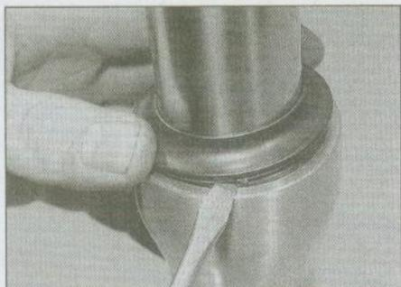
18.3 Prise up the dust seal using a flat-bladed screwdriver
