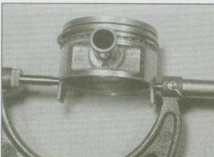
23.13 Measuring the piston diameter at the specified distance from the bottom of the skirt
