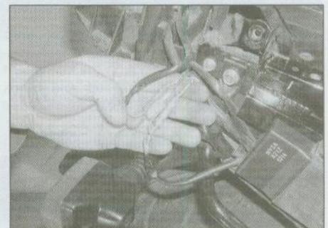
14.5 Wiring connectors for the rear turn signals
