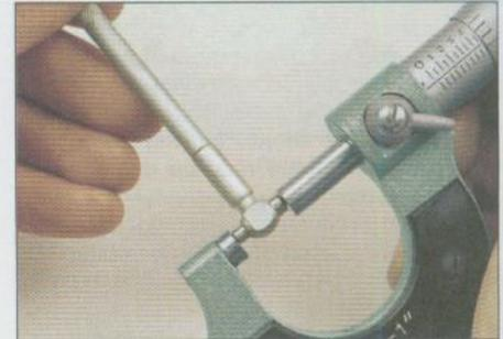
3.8 ... then measure the gauge with a micrometer
