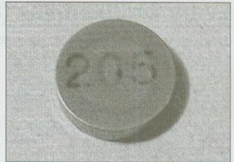
26.13a The shim size should be marked on its face ...
