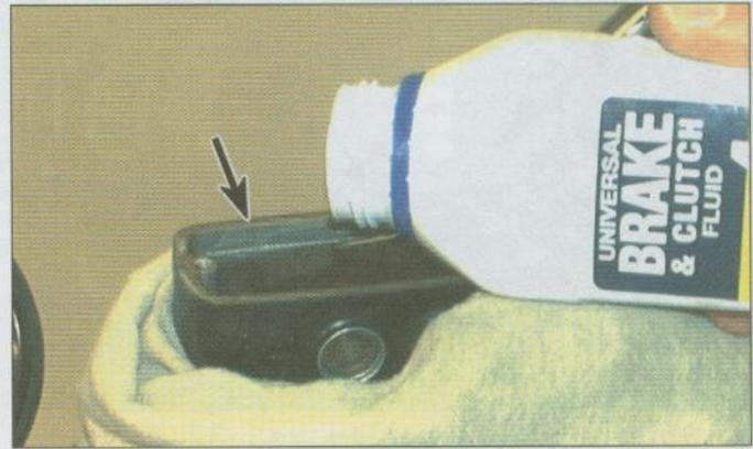
**3** Top up with new DOT 4 hydraulic fluid, until the level is just below the UPPER level line cast on the inside of the reservoir (arrowed). Do not overfill, and take care to avoid spills (see **Warning** above).
