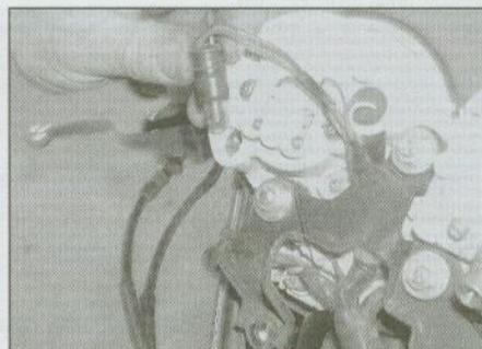
17.4a Pull the bulbholder out of the casing . . .
