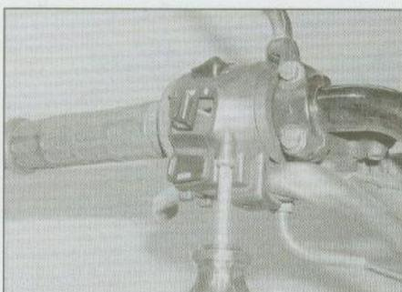
11.3b Remove the screws and split the switch housing
