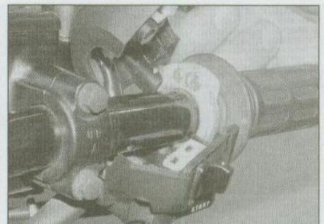
**25.5b** . . . and detach the switch from the handlebar
