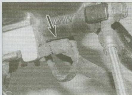
5.4 Brake light switch wiring connectors (arrowed)
