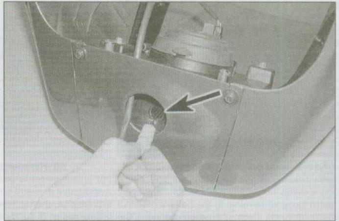
7.24 Bulbholder is a push fit in the headlight shell
