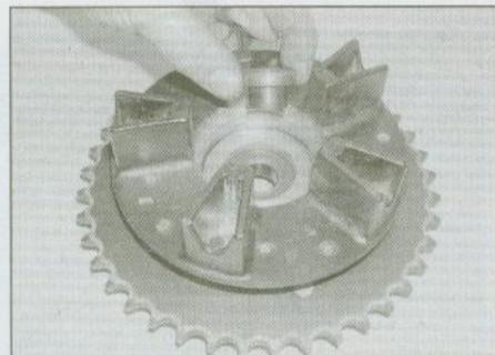
17.34a The spacer fits on the inside of the coupling bearing
