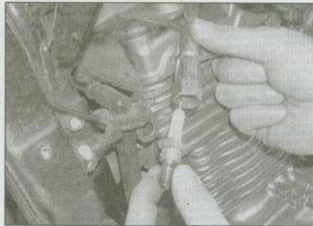
13.5b ... and separate the plug from the tool
