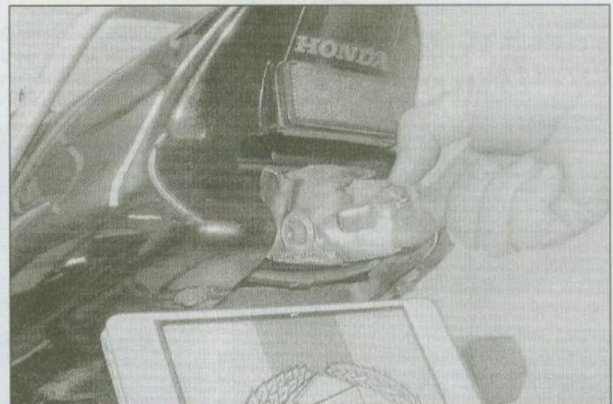
9.2 Twist anticlockwise and pull to remove the bulb
