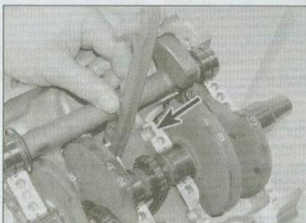
27.3a Note location (arrowed) of front guide blade . . .
