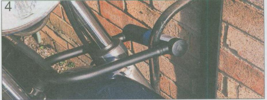
**U-locks can be used to secure the bike to a solid object – ensure you purchase one which is long enough**
