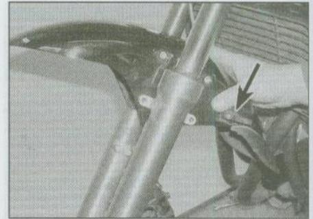
8.2 Lift the mudguard clear of the fork sliders. Speedometer cable guide arrowed
