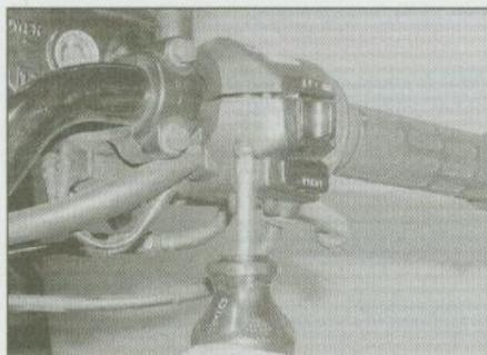
10.7a Separate the halves of the twistgrip housing . . .
