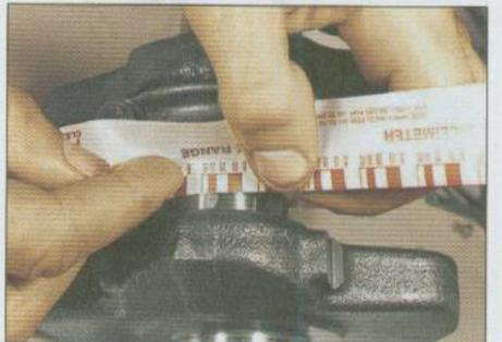
3.16 Measuring the width of the crushed Plastigauge
