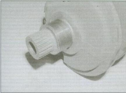
25.6a Inspect the primary gear splines . . .
