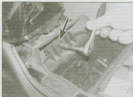
3.2 Battery cover is retained by a single bolt (arrowed)
