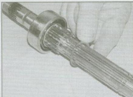
29.18a Slide on the thrust washer ...
