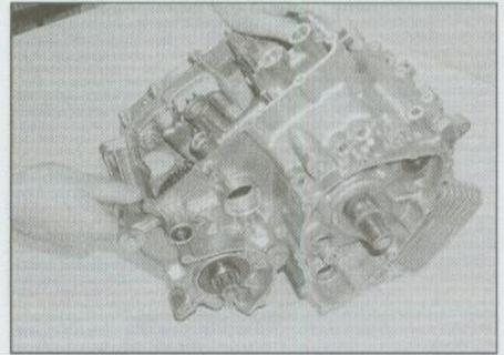
20.17 Carefully lower the lower crankcase half onto the upper crankcase half
