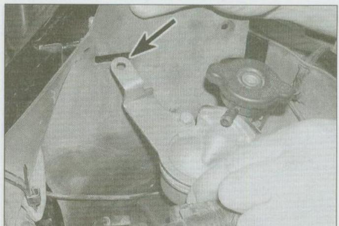
6.11 Thread the bracket through the hole in the rubber shroud (arrowed)
