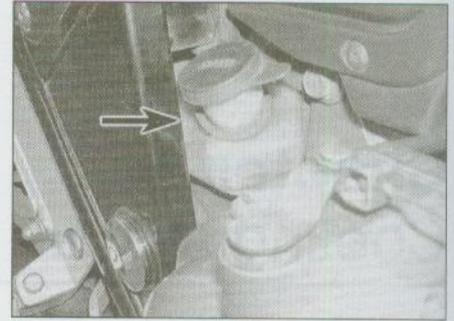
3.1 The coolant reservoir (arrowed) is located under the air filter housing
