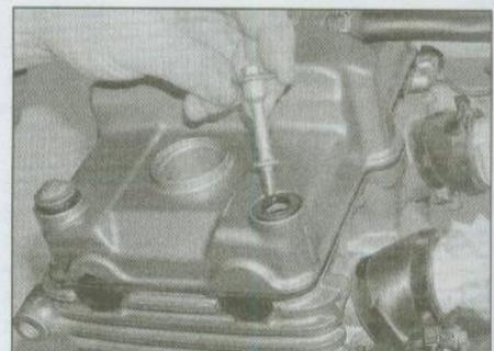
7.9b . . . then install the bolts and tighten to specified torque
