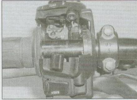
25.5d . . . and detach the switch from the handlebar
