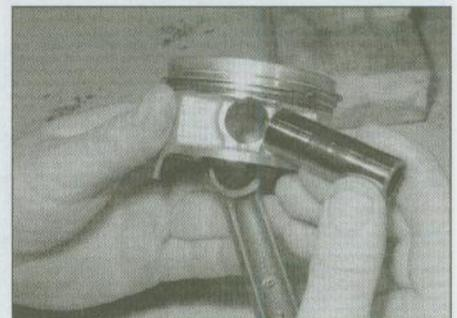
23.4b . . . then push out the pin and remove the piston
