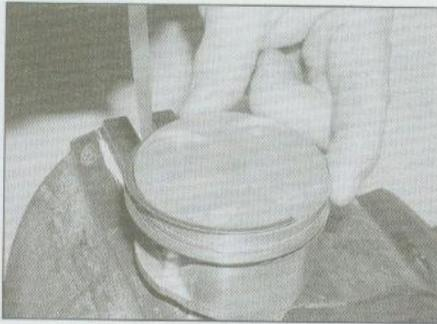
**24.11** Check that the compression rings are the right way up before fitting
