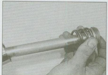
**7.8 Withdraw the damper rod and rebound spring from the tube**
