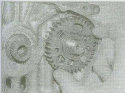
16.9 Install the balancer gear on its shaft
