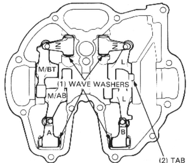
Install each rocker arm in the correct position, referring to the illustration on page 6-18.
