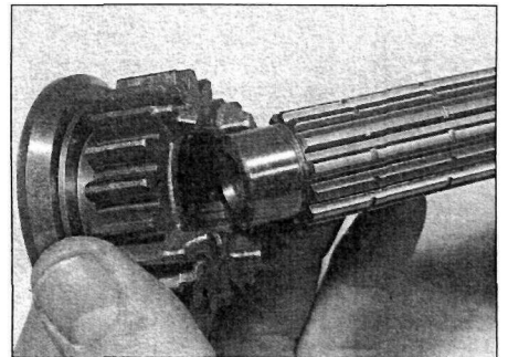
25.17a Install the 3rd gear pinion .
