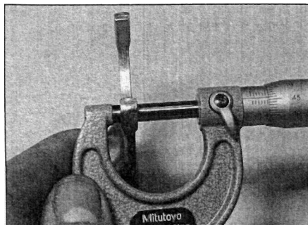
26.3 Measure the selector fork end thickness
