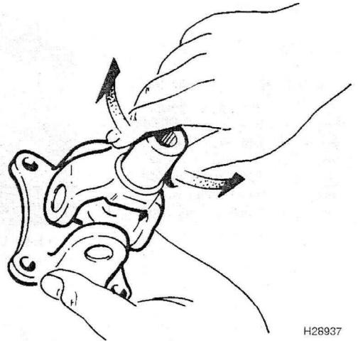
14.7 Checking the universal joint for play in the bearings
