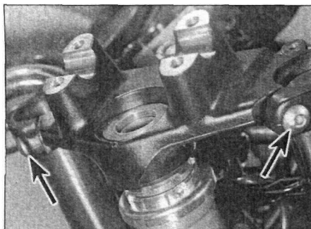
20.7b Slacken the fork clamp bolts (arrows), then lift off the top yoke
