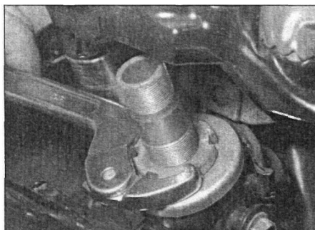
20.9 Adjust the head bearing adjuster nut using a C-spanner
