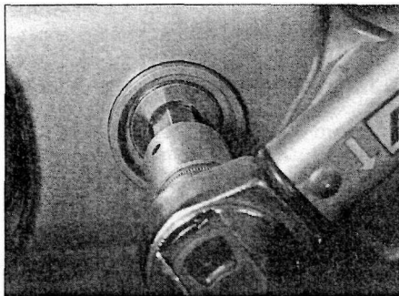
12.12a Tighten the left-hand pivot bolt to the specified torque setting
