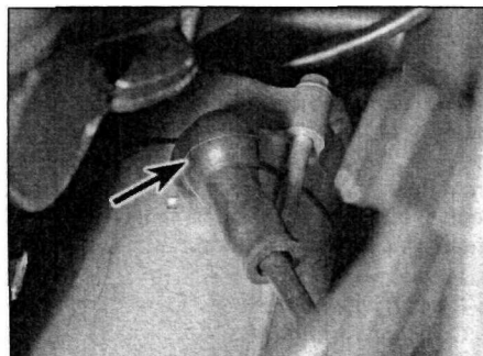
5.13a Pull back the rubber boot (arrow) to expose the starter motor lead securing nut
