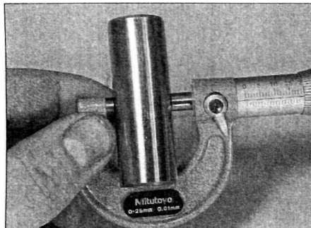
15.13b Measure the external diameter of the pin . . .
