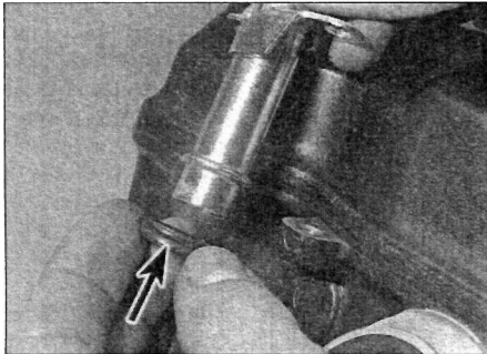
11.25c . . . and withdraw the pipe and its O-ring (arrow)
