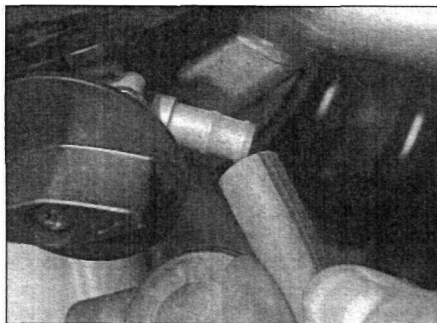
2.9 Connect the fuel hose to the tap
