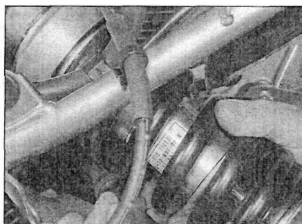
10.7 Remove the shock absorber from the back of the frame
