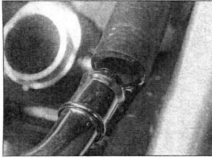
11.25a Detach the coolant hose from the pipe
