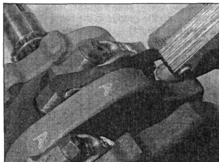
29.2 Measure the connecting rod side clearance
