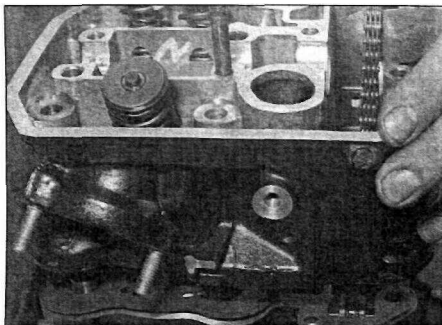
11.36 Carefully lower the cylinder head onto the block
