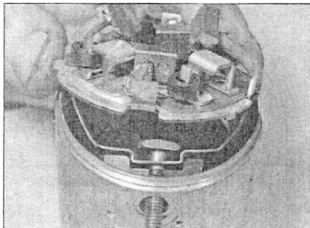
30.16b . . . and install the brushplate assembly and terminal bolt
