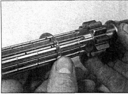
25.16a Install the thrust washer ...
