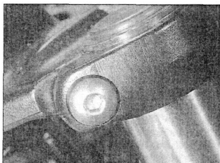
6.4 Top yoke fork clamp bolt
