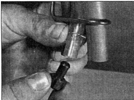
1.1 Remove the plug and allow any deposits to drain from the crankcase breather
