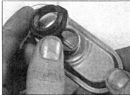
23.15a Fit a new seal to the strainer . . .
