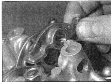
8.8b . . . then remove each rocker arm . . .
