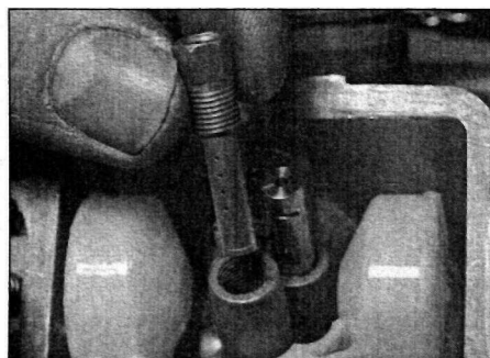
9.4a Install the needle jet
