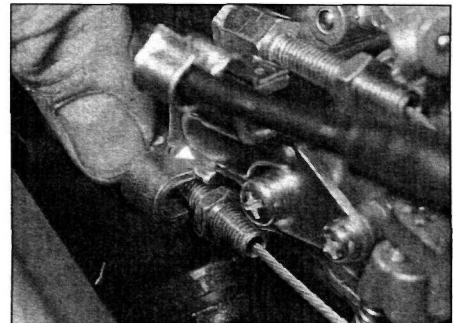
10.8b . . . then secure the cables in the bracket
