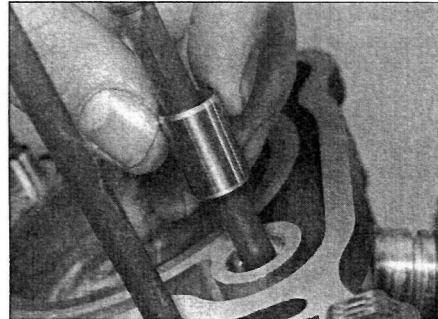
11.34 Install the two dowels over the studs and onto the cylinder block
