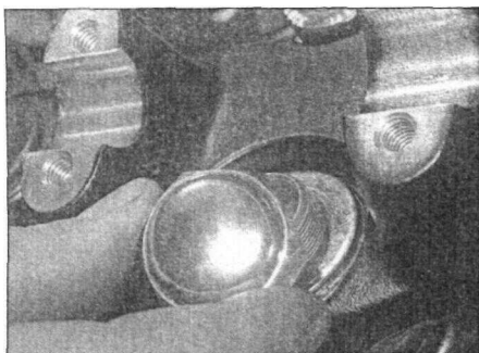
20.7a Remove the steering stem nut and washer
