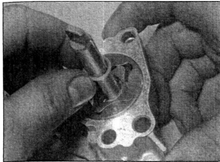
23.14d Install the thrust washer over the shaft and onto the inner rotor
