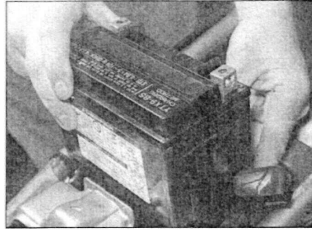
3.1c Lift the battery out of its case
