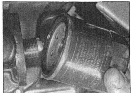
11.7 Apply a smear of motor oil to the sealing ring of the filter on installation
