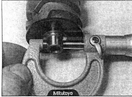
26.7 Measure the selector drum journal diameter
