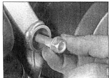
5.24b Unscrew the nut and withdraw the bolt
