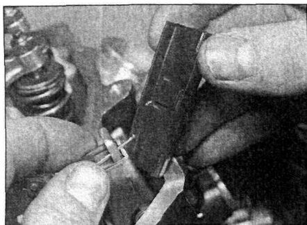
10.7 Make sure the rubber cushion is correctly installed
