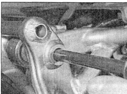
10.6b . . . and remove the bolt
