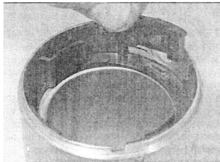
30.16a Locate the insulator in the housing . . .
