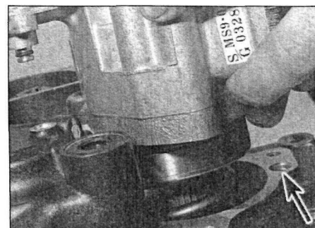
24.17c . . . fits into its hole in the crankcase (arrow)
