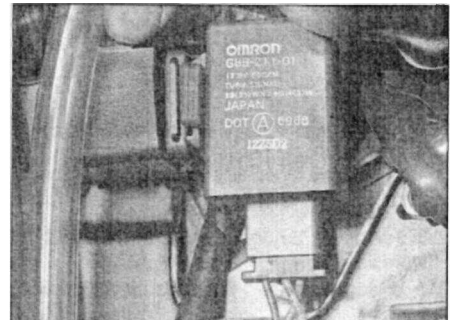
13.3 Turn signal relay location
