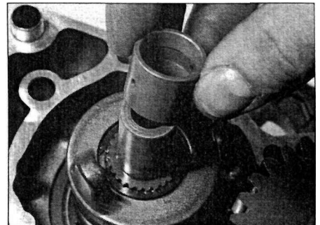
24.2c ... and the bushing from the output drive shaft
