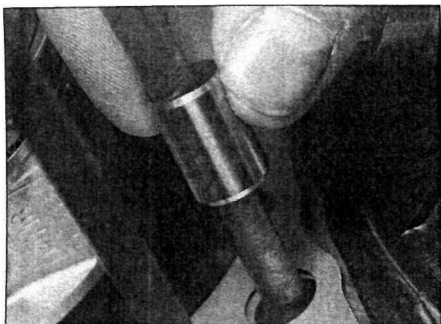
14.16 Install the two dowels over the studs and into their crankcase recesses
