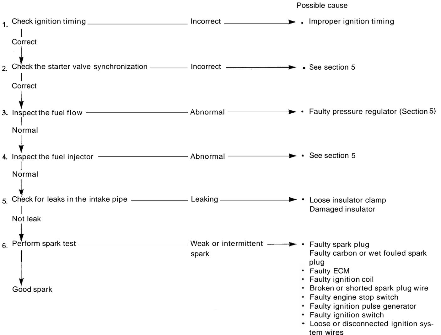
**POOR PERFORMANCE AT HIGH SPEED**
