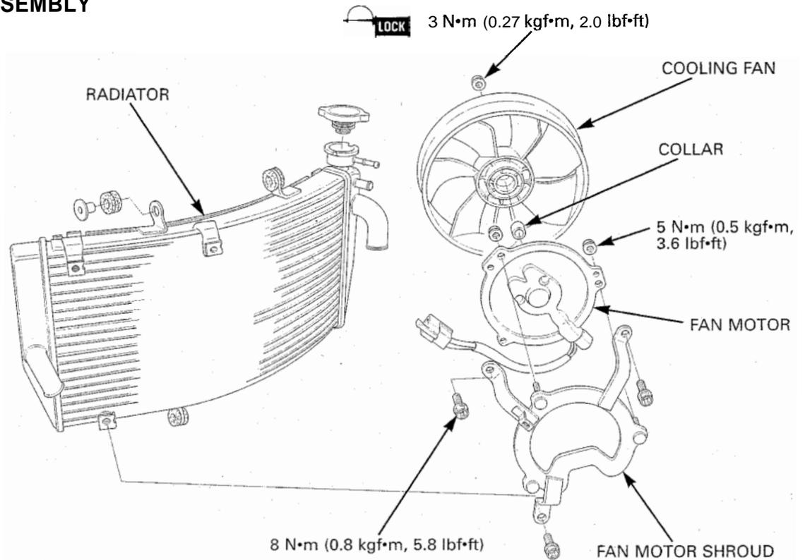
Install the fan motor onto the fan motor shroud with the drain hose facing as shown. Tighten the flange nuts to the specified torque.
