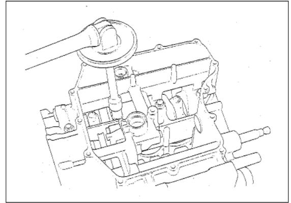
Remove the 9 mm bolts and lower crankcase. Measure the compressed plastigauge on each journal.
