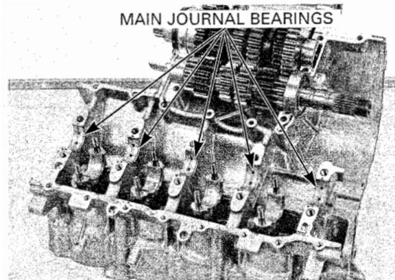
Wipe the oil from the bearing inserts and journals. Reinstall the upper crankcase's main journal bearing inserts, then carefully lower the crankshaft in place. Put a piece of plastigauge on each journal.
