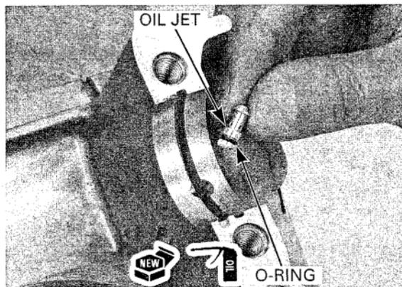
*The bearing tabs should be aligned with the grooves in the case.*
