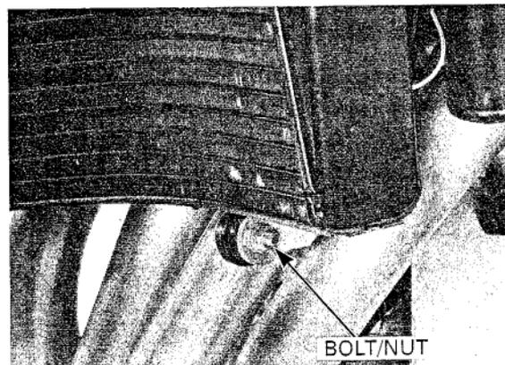
Remove the radiator upper mounting bolt and washer.
