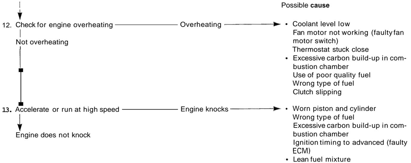
**POOR PERFORMANCE AT LOW AND IDLE SPEED**
