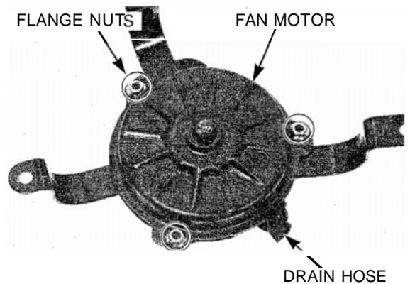
Install the distance collar onto the fan motor shaft.
