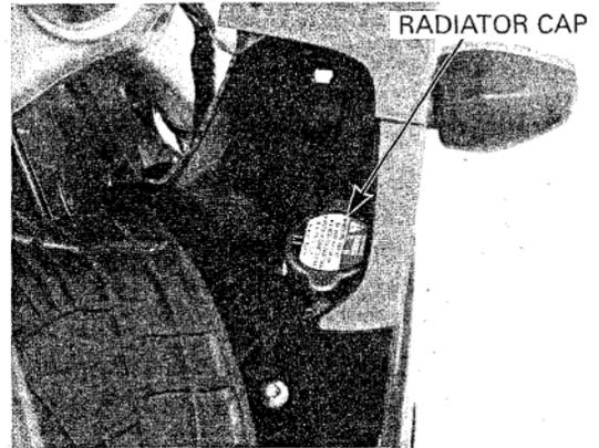
Test the coolant specific gravity using a hydrometer (see below for "Coolant gravity chart"). For maximum corrosion protection, a 1:1 solution of ethylene glycol and distilled water is recommended (page 6-4). Look for contamination and replace the coolant if necessary.
