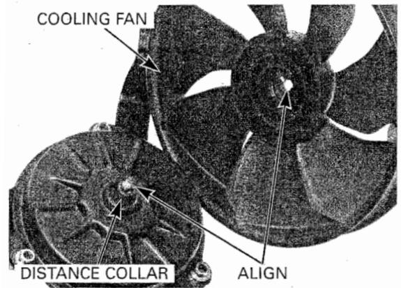
Apply a locking agent to the cooling fan nut threads.
