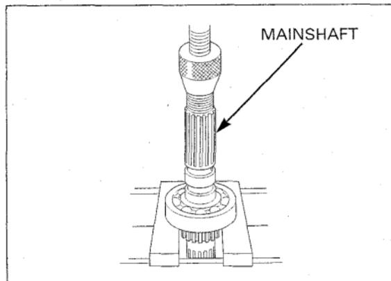
Install a new mainshaft bearing onto the mainshaft by pressing the mainshaft bearing inner race using the special tool.
