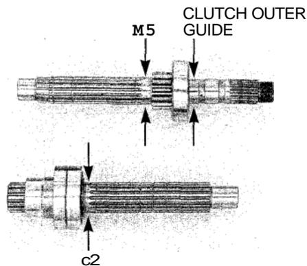
*Do not try to remove the countershaft bearing from the shaft. If the bearing is worn or damaged, replace the countershaft as an assembly.*
