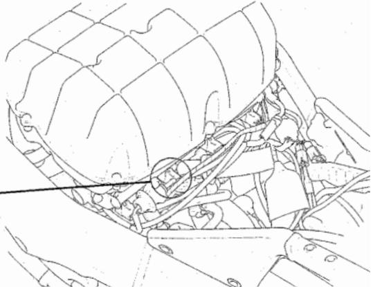
Connect the No.2 injector 2P connector.
