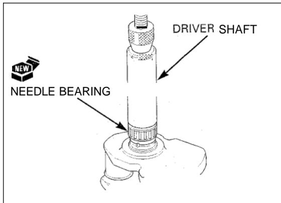
If the special tool is not available, prepare a suitable collar, washer and 10 mm flange bolt (example; fly-wheel bolt) for the bearing installation.
