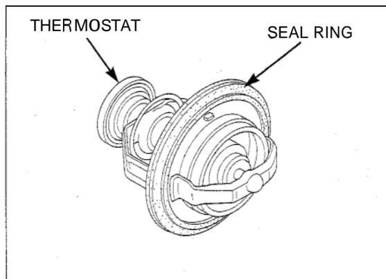
Heat the water with an electric heating element to operating temperature for 5 minutes. Suspend the thermostat in heated water to check its operation.
