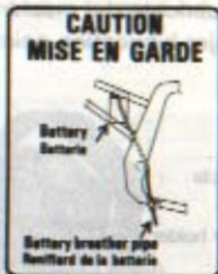
The battery is located under the seat. The solution level must be kept between the UPPER and LOWER level lines at all times. If the solution level is below the LOWER level line, add ONLY distilled water up to the UPPER level line. NEVER use tap water.
