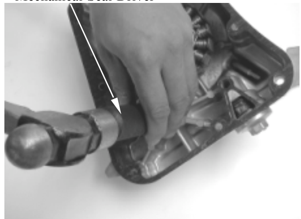
Mechanical Seal Driver
