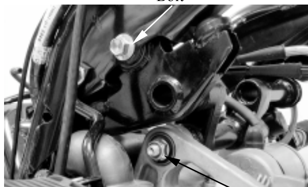
Engine Mounting Nut
