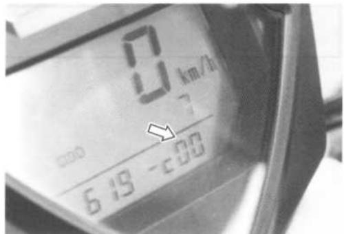
**MALFUNCTION CODE AND DEFECTIVE CONDITION**
