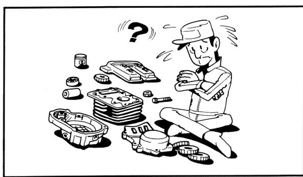
3. During the engine disassembly, clean all parts and place them in trays in the order of disassembly. This will speed up assembly time and help assure that all parts are correctly reinstalled in the engine.
