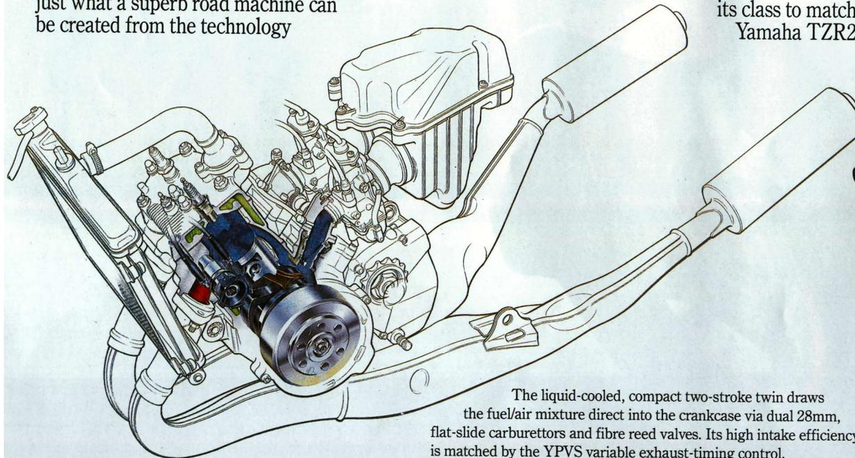
The liquid-cooled, compact two-stroke twin draws the fuel/air mixture direct into the crankcase via dual 28mm, flat-slide carburettors and fibre reed valves. Its high intake efficiency is matched by the YPVS variable exhaust-timing control.
