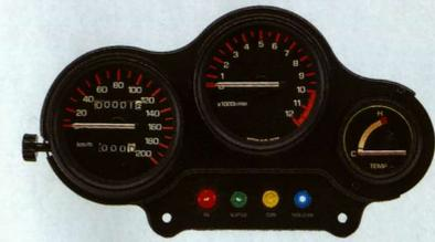
Focal point of the racer-styled instrument panel is the highly-visible tachometer with white face and black numerals. It is flanked by the speedometer and coolant temperature gauge.
