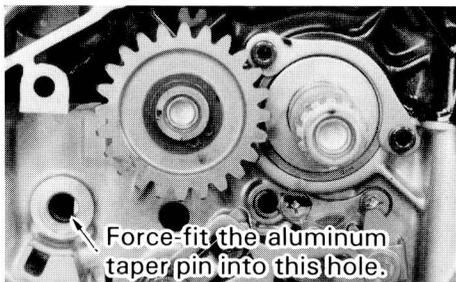
Force-fit the plug until it is flush with the crankcase surface.
