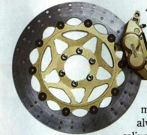
The racing-quality front disc brake uses a 320mm-diameter rotor, drilled to compensate for heat expansion and "floating" on its mountings so that it always runs true in the caliper for maximum pad
