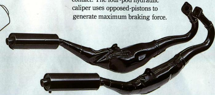
The TZR250 exhaust system uses genuine racing-type "expansion chambers", with no baffling in their centre section, that are a key factor in the machine's high power output. Baffling in the tail-pipe, plus separate mufflers, keeps noise level down, however.
