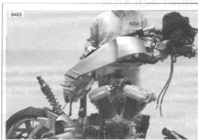
Figure 2-82. Lift Frame Off Motorcycle
