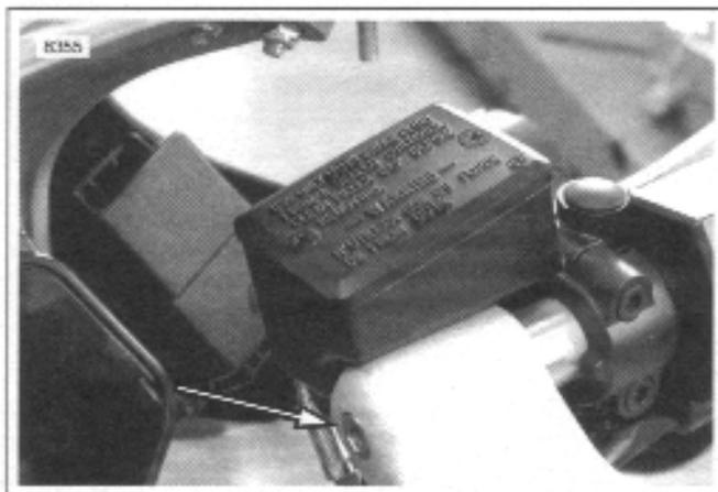
Figure 2-96. Handlebar Clip-on Mounting Fasteners (right clip-on shown)
