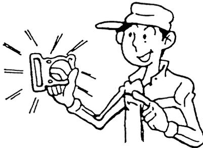
3. When disassembling the machine, keep mated parts together. They include gears, cylinders, pistons, and other mated parts that have been "mated" through normal wear. Mated parts must be reused as an assembly or replaced.
